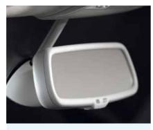
Automatically dimming rear view mirror. Standard on the Executive, the rear view mirror features photocell control. It dims automatically when the headlights of following vehicles are too bright.
